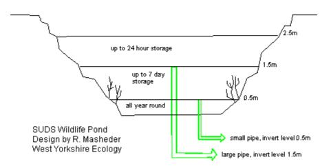
Figure 65 - an indicative design to demonstrate how a SUDS detention pond can be utilised for the dual purpose of wildlife pond habitat and as a receptor site for runoff from roofs
