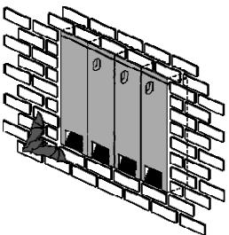
Figure 63 - four Schwegler bat tubes linked together within the wall of a building.
