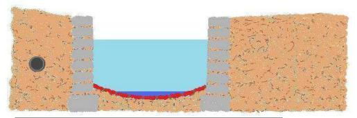
Figure 34a – current brick-lined stretch of Bradford Beck
