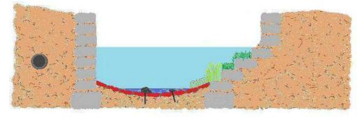
Figure 34b – boulders on bed to slow flow and re-grading of eastern bank
